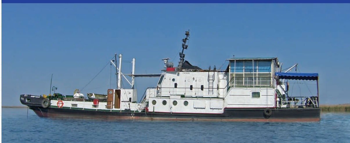
Fluvial and coastal research vessel "Istros": displacement - 147,8 t, scientists - 10 persons, 3 laboratories, endurance - 900 km
