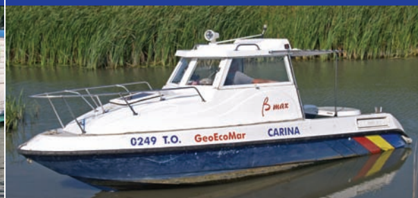
Research - surveillance motorboat "Carina": length - 6 m, 6 seats, 150 hp, diesel motor
