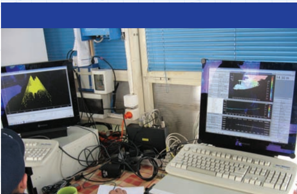
"Sea Beam 1050 D" ELAC Naautik multibeam bathymetric system
