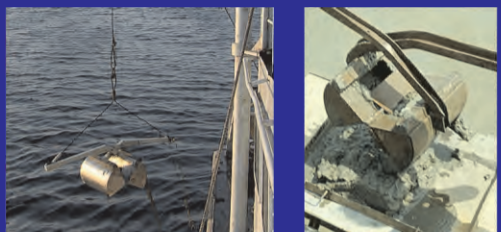
Fig. 2. "Van Veen" grab sampler.
