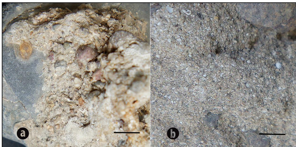
**Plate 1. a)** Dredged marine conglomerate (note the remnants of a bryozoan in the upper right corner of the slide); **b)** Infra-loessic conglomerate collected onshore at the base of the Nantois cliff. Black scales: 1cm.
