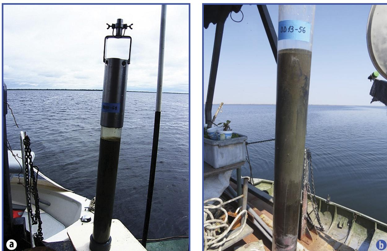
Fig. 2. Hydro-Bios corer (a), used for taking the short cores, and a transparent plastic tube with sediment inside (b).
