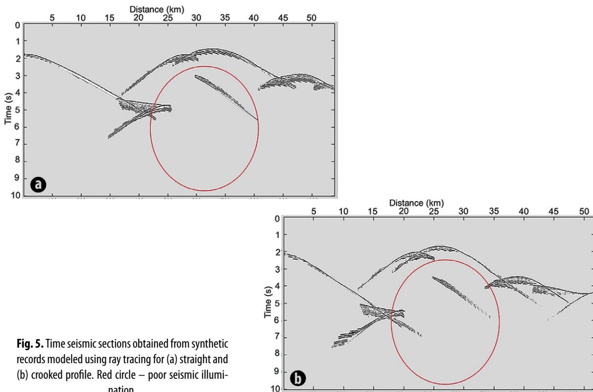
**Fig. 5.** Time seismic sections obtained from synthetic records modeled using ray tracing for (a) straight and (b) crooked profile. Red circle – poor seismic illumination.
