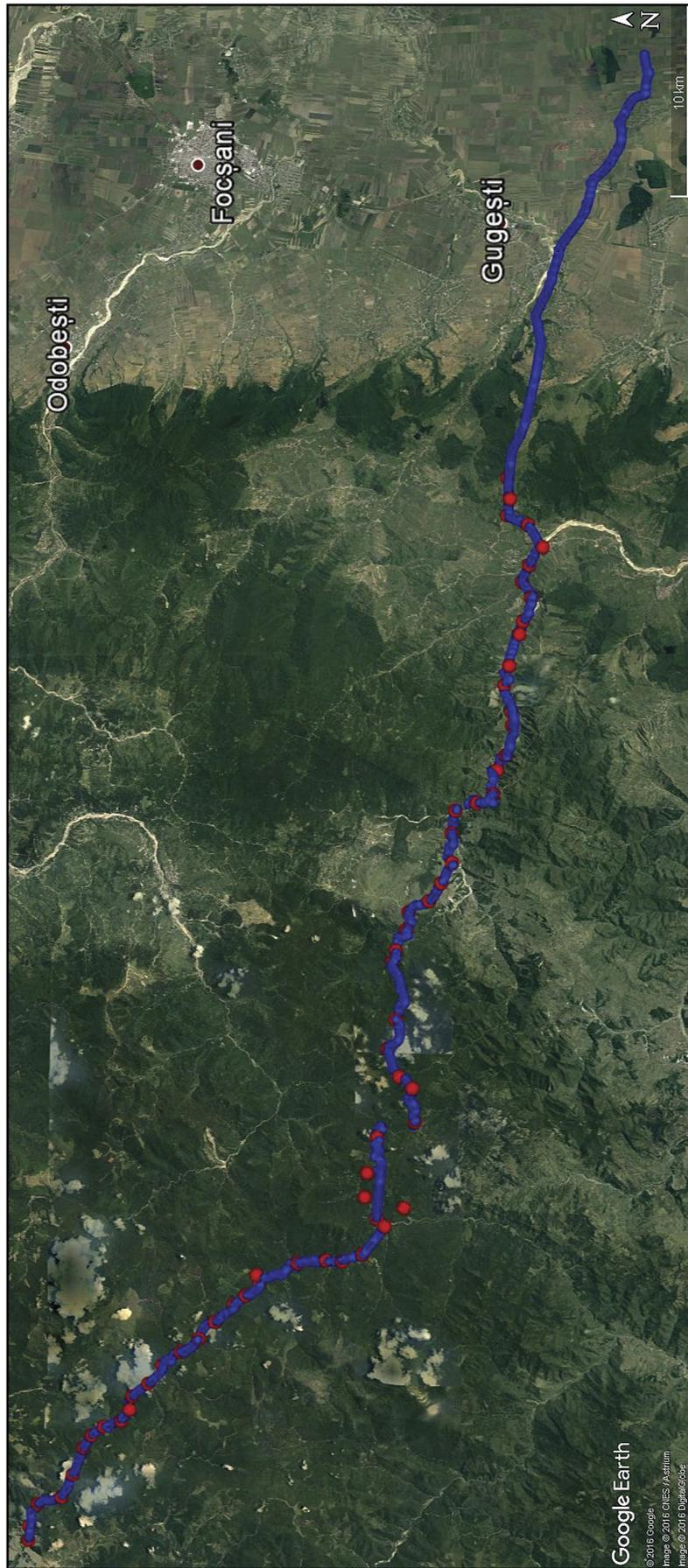
**Fig. 2.** Map showing the positions of the receivers and sources on the seismic profile; blue – receivers, red – sources. Source map: <http://maps.google.com>.
