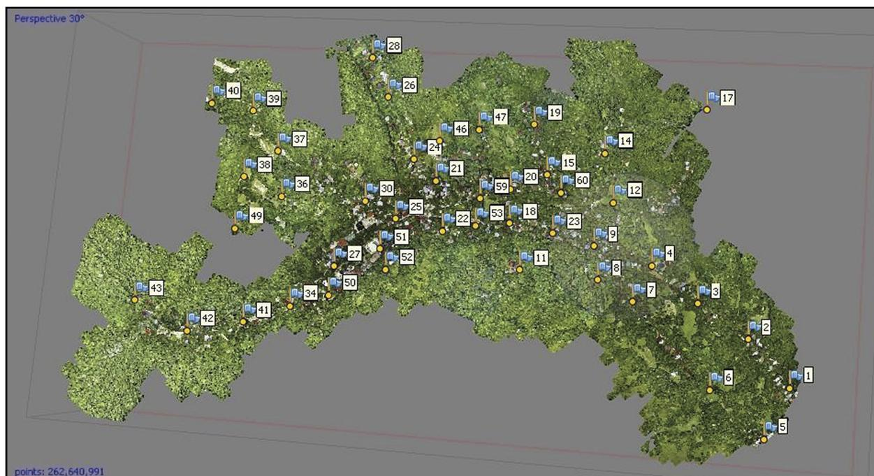
**Fig. 2.** The dense could points and the entire set of landmarks (with numbers) used as control points.
