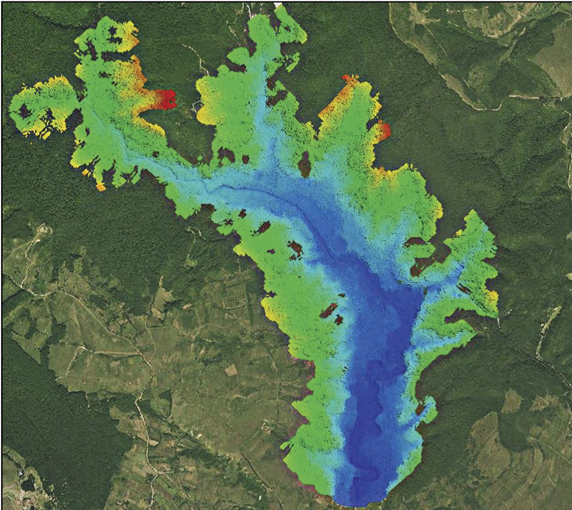
**Fig. 4.** DEM (Digital Elevation Model) overlapped on a satellite image of the area (downloaded from the World Imagery server affiliated to Global Mapper), the representation and visualization being in the form of pseudo-colors (using blue for the lowest elevations and red for the highest elevations).
