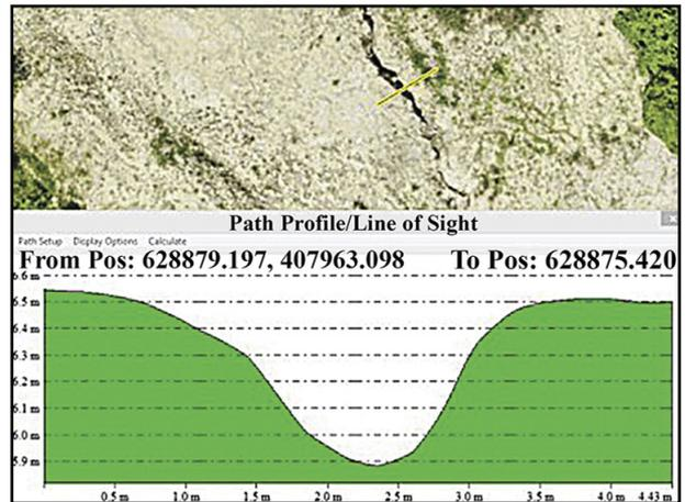
**Fig. 7.** Topographic profile of a fracture located in the outcrop, mentioned in the previous figure, generated in Global Mapper.
