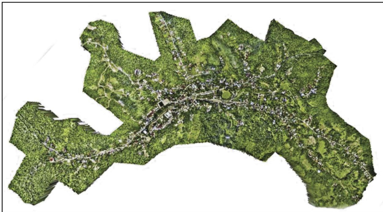
**Fig. 11.** The orthophotomap representing the geometrically corrected image referenced in the Stereo70 projection system.
