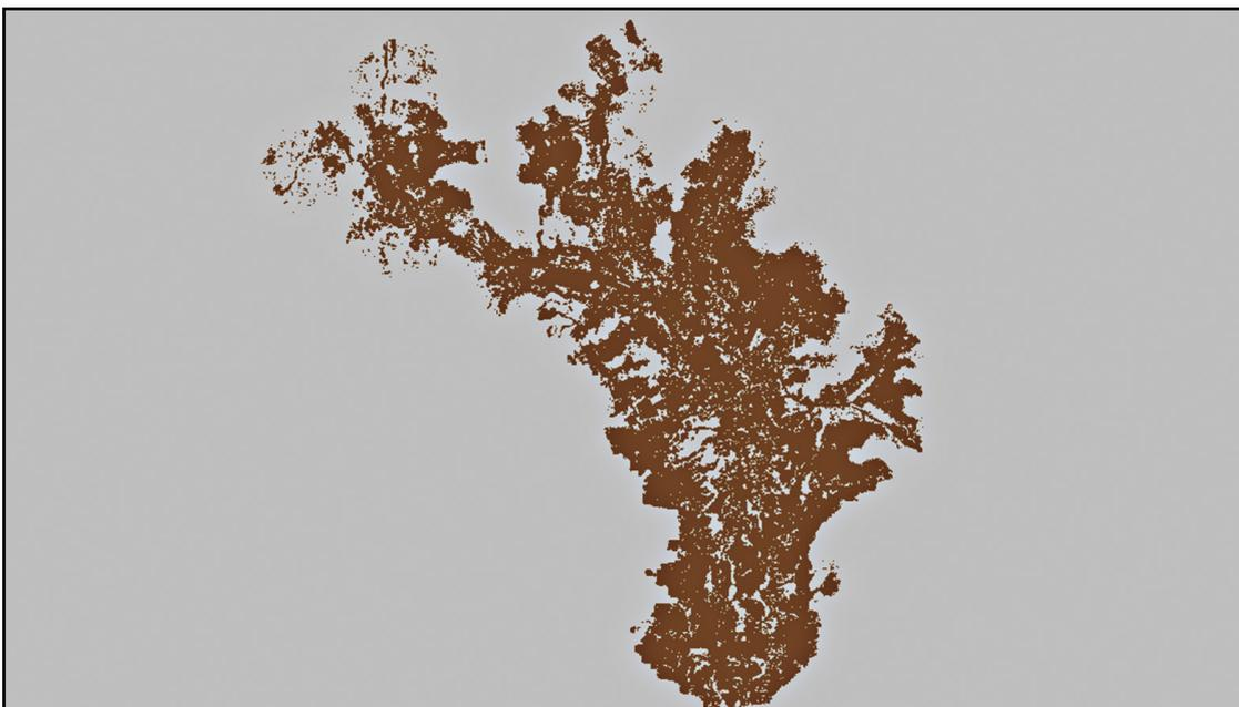
**Fig. 5.** The classified point cloud generated in Global Mapper, in which the brown parts represent the ground class and the grey areas are unclassified.
