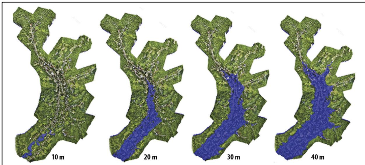
Fig. 9. Flood simulations and floodplain maps, from left to right; the level of water rises 10 m each.
