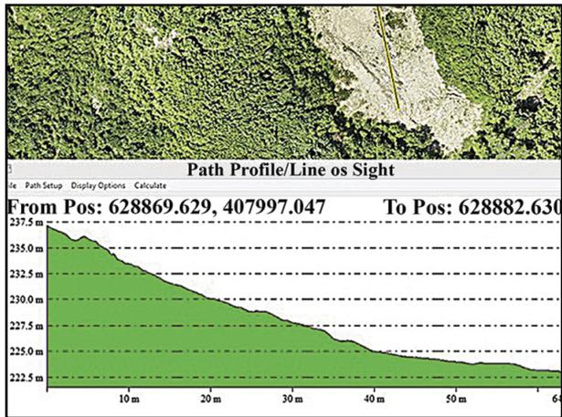
**Fig. 6.** Topographic profile of an outcrop (situated in the north-eastern part of Sărata Monteoru) generated in Global Mapper.
